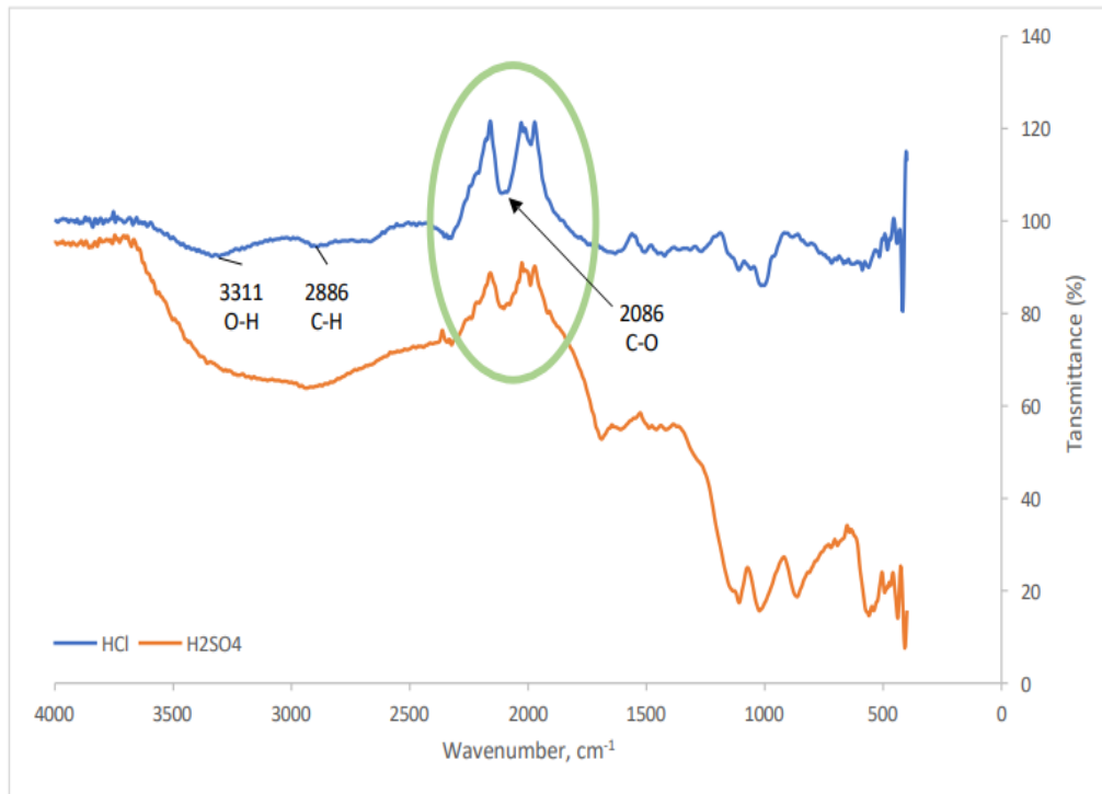
Figure 7: Acid hydrolysis of H 2 SO 4 and HCl under FTIR Spectra
